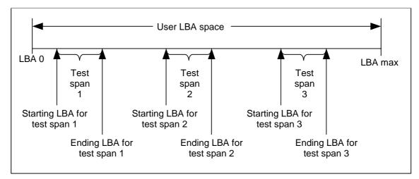
Selective self-test test span example
